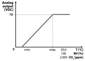
The output voltage starts to rise from 0 VDC at minimum sensor range and reaches 10 VDC at maximum sensor range.
