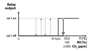
The relays switch on at setpoints selected via the trimmers and switch off with fixed hysteresis 2  $^{\circ}$ C, 5  $^{\circ}$ RH, 100 ppm.
