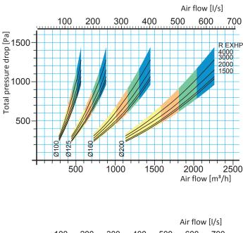
The black line shows the pressure drop for the arm when in the same position as in the design above. The area in the diagram shows the pressure drop at normal use. The field's tints show air velocity in the extractor according to below.
