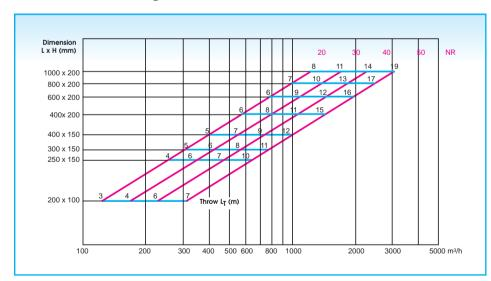
Valid for supply only. See diagram p. 1 050 for exhaust. Throw factor is based on a  $v_R$  of 0,17 m/s in the occupied zone. See p. 1 050 for a detailed selection and other dimensions.
