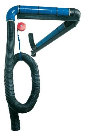
The Fumex balancing block solution, type ASA without pivoting arm, is equipped with hose, balancing block and suspension belt. The extractor is mounted hanging from the ceiling or other high location. For wall mounting, wall bracket ASA V is available.
